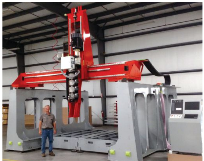
A massive plastic-extrusion additive manufacturing system is in development by Thermwood, a traditional CNC equipment manufacturing company, is pictured. Image courtesy of Thermwood.
