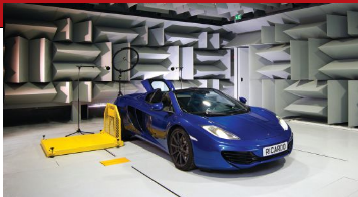
RIGHT: Ricardo's Vehicle Anechoic Test Facility (VATF) includes a "rolling road" integrated chassis dynamometer. Image courtesy of Ricardo.
