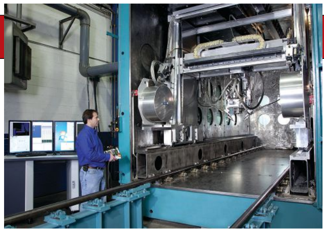
Sciaky's EBAM 300 series metal 3D printer can produce parts that are 19 feet long, 4 feet wide and 4 feet high. Image courtesy of Sciaky.
