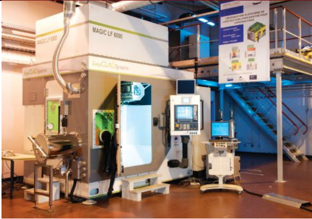
MAGIC LF 6000 additive manufacturing system from BeAM. The company's CLAD technology creates or repairs parts with laser-melted metal powders. Image courtesy of BeAM.
